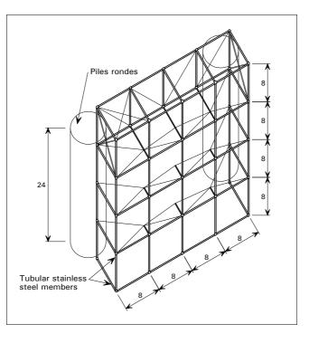
Each 8 m member was cast in four 2 m long sections which were butt welded together. The tubes were machined on a lathe along their length giving a striated appearance (Figure 4). A relatively roughened surface finish was sought to blend with an orange-peel finish on the nodes.
