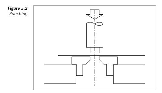
Profiles can be punched out of stainless steel sheet using NC (numerically controlled) punching machines. In this process the workpiece is held under a repeating punch, using a clamp that repositions the workpiece between every punch stroke.
