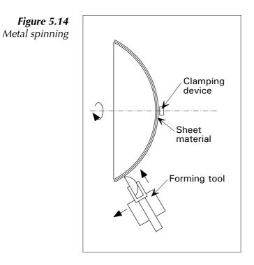
Tooling is inexpensive, but the process is labour intensive, making it most suitable for low volume production runs. The range of shapes that can be achieved is limited (all objects require one axis of rotational symmetry).
