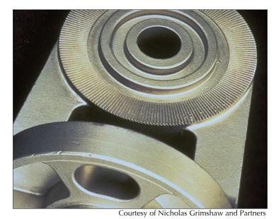
*Figure 7* Prototype stages of cast stainless steel elements (foam, wood, wax pattern and final casting)
