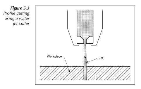
Water cutting does not heat, distort or change the properties of stainless steel, and is safe to use in environments where flame cutting would be hazardous (*e.g.* in fire risk zones). The use of water jet cutting is increasing, and costs are falling.
