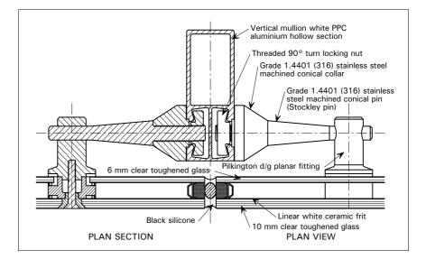
*Figure 4* The Stockley pin assembly
