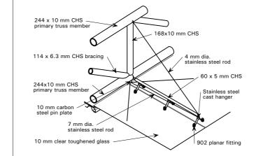
The 3 m wide canopy is suspended using stainless steel tie rods and turnbuckles, and similar castings to those used in the main roof.
