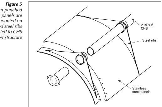
Custom-punched mounted on pressed steel ribs bolted to CHS support structure
