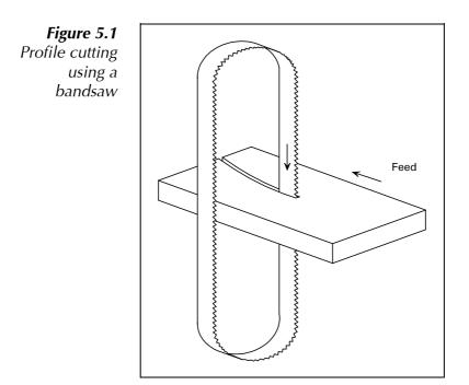
The technique is better suited to sweeping profiles than those with tightly rounded corners, although difficult features can be achieved by other profiling methods after the basic shape is cut. The hardness of stainless steel requires the use of alumina or silicon carbide coated blades.
