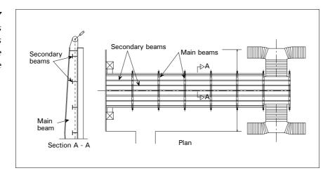
$140 \times 10$  mm stainless steel CHS are used as hangers for the mezzanine. The main beam is pin connected to a stainless steel machined head, which is welded to the tubular hangers (Figure 8). Machined stainless steel hangers provide the connection to the roof via 30 mm thick stainless steel plates anchored by grouted hammer head bolts (Figure 9).
