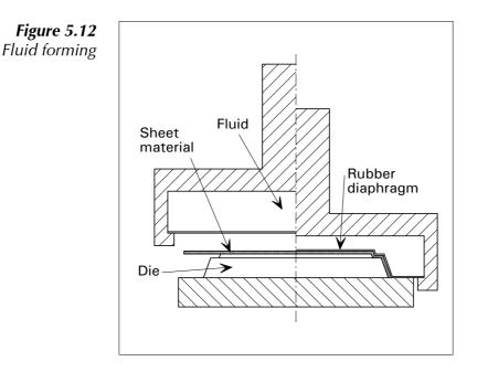
Considerable savings can be made for low to medium volume production runs as the rigid die does not have to exactly match an opposing die, and is not subject to high impact stresses. Rigid dies can therefore be made from a range of easily worked materials such as plastics, composites, timber, aluminium, softer grades of steel and special re-usable alloys.
