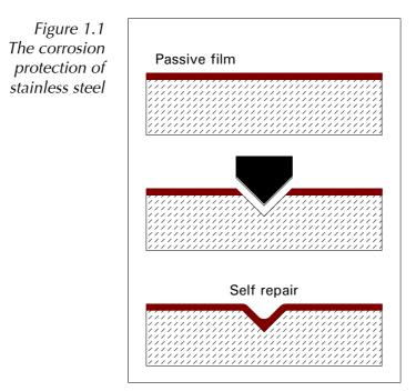
Many grades of stainless steel are available, each with different mechanical and physical properties. Generally, corrosion resistance increases with the chromium content of stainless steels.
