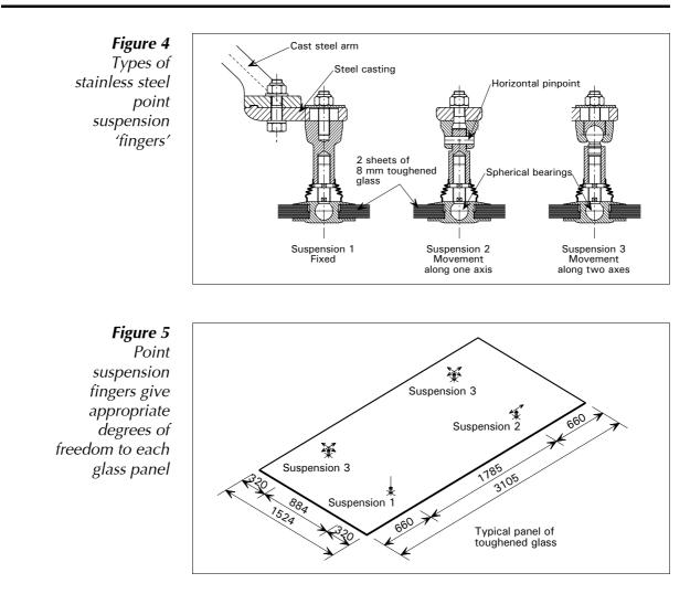
The point support fingers are CNC (Computer Numerically Controlled) machined from grade 1.4401 (316) stainless steel. They are isolated from the carbon steel cast arms by a 0.5 mm dense polymer composite foil, washers and bushes. Stainless steel was used for its durability and corrosion resistance and to eliminate any need for repainting close to the glass.
