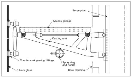
Within the glass enclosure, the surge pipe is clad using 3 mm stainless steel sheet with a mirror finish (Figure 6) which is sectioned to visually reinforce the vertical calibration of the tower.
