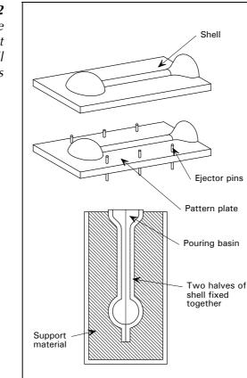
Compared to sand casting, the resin casting process gives higher degrees of accuracy, and better surface finishes are possible by using fine grained sand. Less finishing tends to be required than for sand casting and this may compensate for higher mould costs. Where components are symmetrical, one pattern plate may be used for both halves of the mould.
