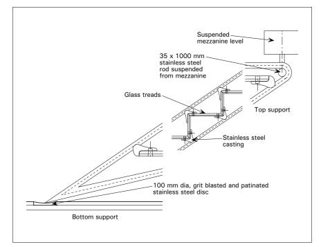
Techniques Laser cutting Spinning Tube bending Sand casting Brushed finish Welding
