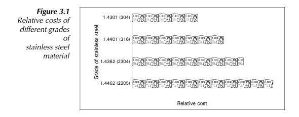
A stainless steel component may cost slightly more to fabricate than an identical carbon steel component because:
