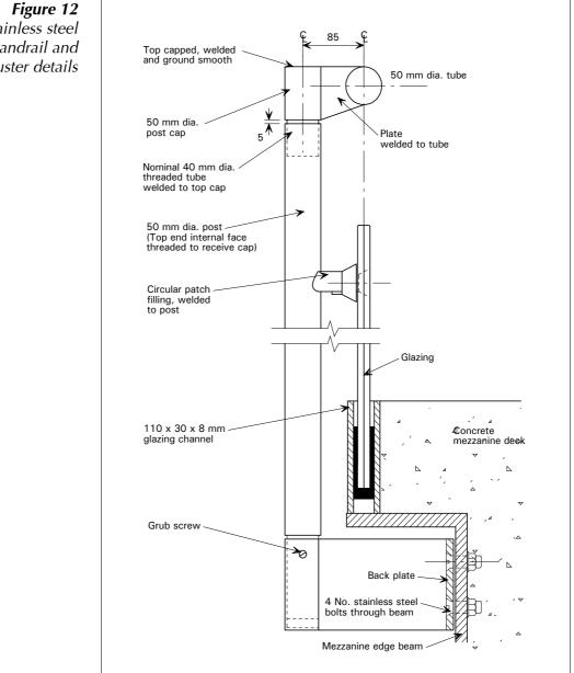
Stainless steel handrail and baluster details
