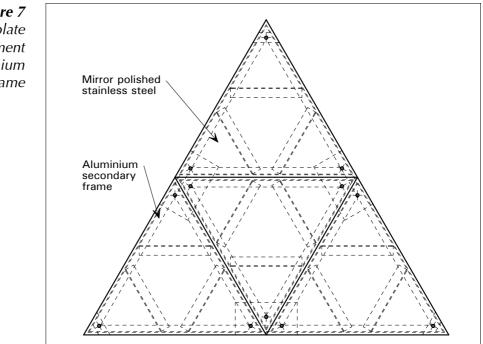
*Figure 7 Triangular plate arrangement onto aluminium frame*
